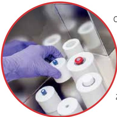
One aim of the QC-Cubicle is to increase the safety of the users. To reach this goal we have increased the radiation protection with specific shielding and an improved environmental control. Additional lead shielding on sensitive parts and some small handling tools reduce the risk of irradiation during the QC and the sample preparation.
