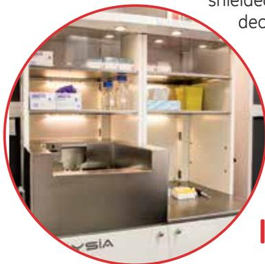
The module is delivered with some special sample holders, small shielding and working tools to facilitate the work and to minimize the hands-on time. The automatic door opener for the waste makes the work smooth and easy.
