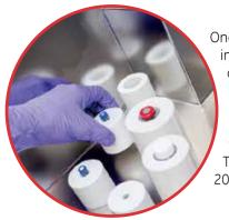
One aim of the QC-Cubicle is to increase the safety of the users. To reach this goal we have increased the radiation protection with specific shielding and an improved environmental control. Additional lead shielding on sensitive parts and some small handling tools reduce the risk of irradiation during the QC and the sample preparation.
