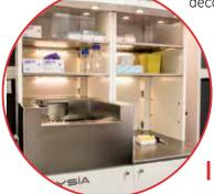
The module is delivered with some special sample holders, small shielding and working tools to facilitate the work and to minimize the hands-on time. The automatic door opener for the waste makes the work smooth and easy.
