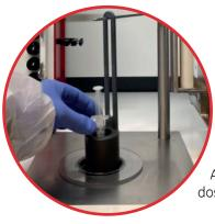
To lower the background noise, the entire dose calibrator compartment has a 10mm lead wall. Its dimensions allow the integration of available dose calibrators (i-Dose, Veenstra, Capintec, Atomlab,...).
