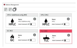
GINA X is able to control several chromatography systems at the same time. With one PC or user access point you can control several HPLC's or other chromatography systems such as a GC or our miniGITA. The user-friendly interface allows a simple overvieuw of all available systems and makes the lab management easier.
