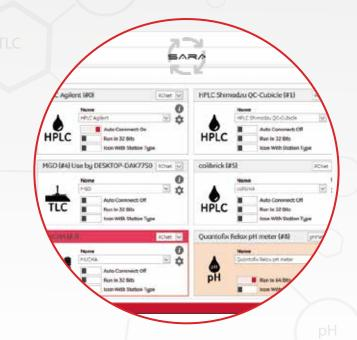
SARA is a central data recording and reporting system for all quality control data for production batches. Authorities require complete documentation of radio-pharmaceutical production, covering raw materials, production process, quality control and aseptic processing.
